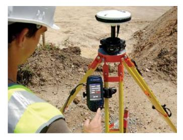
Locating and surveying hard-to-find points is a snap with the navigation and data collection capabilities of ProMark3. After navigating to a point using the unit's base map, transitioning to survey mode requires only a single keystroke.
