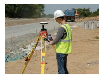
Stop & go surveys are simplified with ProMark3. The portability and the user-friendly interface enable a one-man crew to perform quick and reliable surveys.
